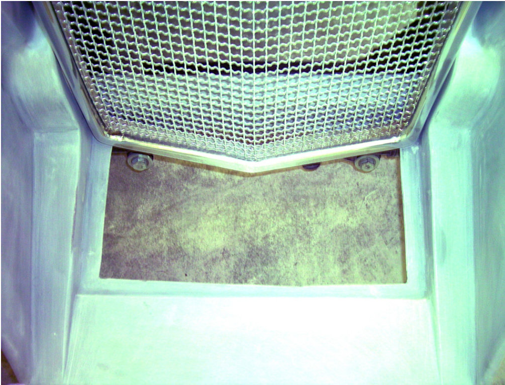
November 2004 - The Splash pan in front of the radiator grill was cut out and will have a metal louvered panel installed.
