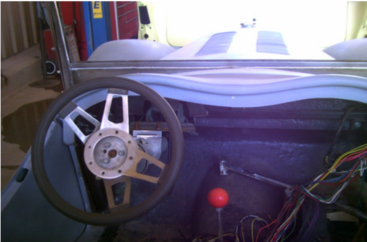
Tilt-steering wheel assembly in place (need to buy a new wooden wheel). Wires from harness awaiting connection to dash instruments.
