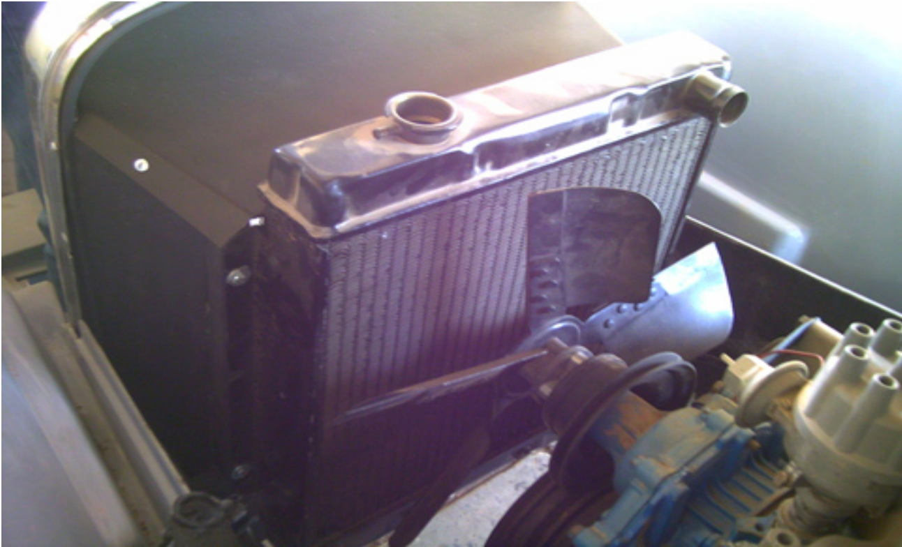
Mustang radiator and shroud installed. Mechanical fan in place on front of engine.
